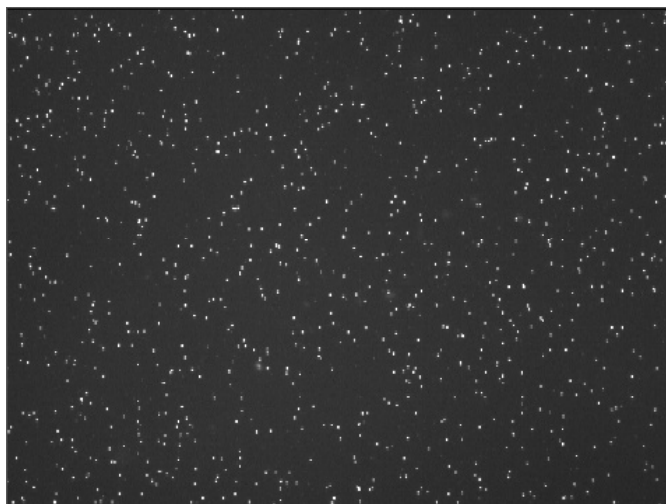
Image 1: Typical NucleoCounter ® image when viewed in NucleoView Software. Cells are shown as light dots. Cells have been treated with Reagent A100 and Reagent B before analysis in the NucleoCounter Instrument.
