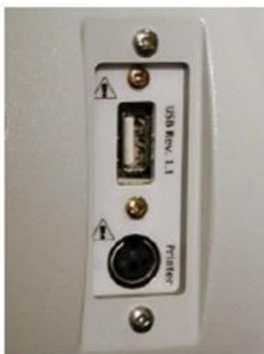
Figure 1 Location of the Printer output on the NucleoCounter ® SP-100 ™ (lower connector).
