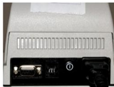
Figure 2 Location of the Serial connector on the PCNEOS printer (to the left).
