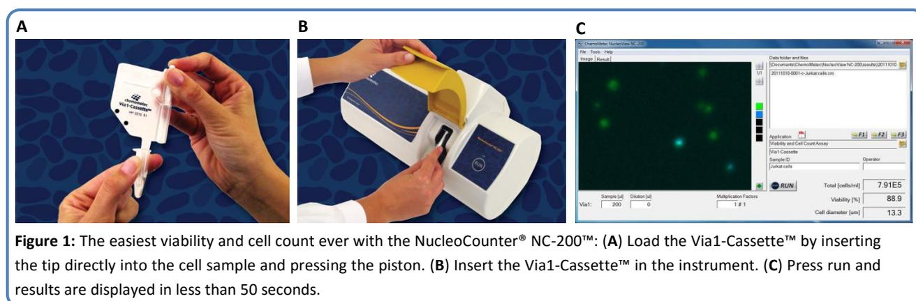
viability. The first dye, Acridine Orange (AO) stains the total cell population, whereas the second dye, DAPI, only stains the non-viable cells. As the cells are stained inside the Via1-Cassette™ no pretreatment is required for this type of analysis.
